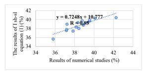
Figure 4: Correlation between the results of the numerical studies and the proposed equation (1) for the Shadow-Sunlit index.
