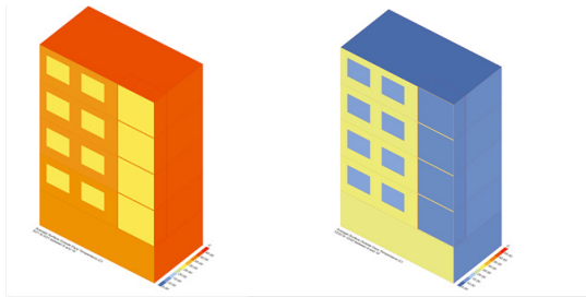
Figure 6: Average temperature of the surfaces in summer solstice (right) and winter solstice (left) of model number one between 6:00 and 7:00 p.m.
