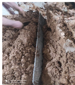
Figure 7: Placing the retaining wall under the dam model
