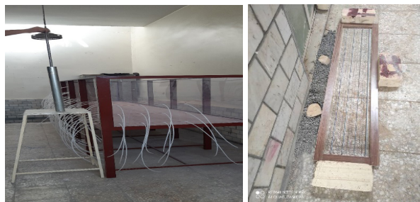
Figure 6: Transparent chamber of the earth dam model and the water retaining wall formwork
