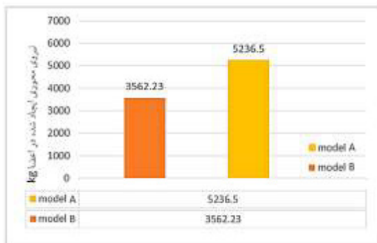
Figure 10: Comparison of the axial force generated at the foot of the column in the SMA model with materials (A) and the SMA model without materials (B)
