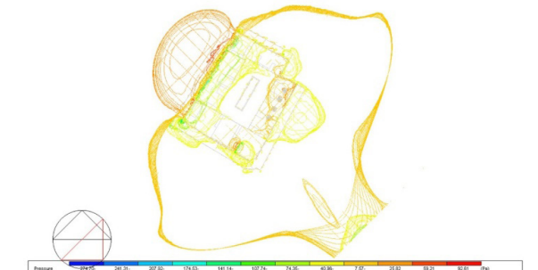
Figure 10: Simulation of the effective pressure due to the wind in the Lariha house (plan)
