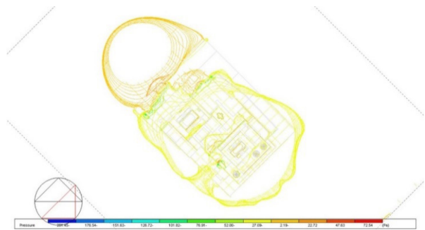
Figure 7: Simulation of effective pressure due to wind in Golshan House Figure 8- Simulation of effective pressure due to wind in Golshan House (plan)
