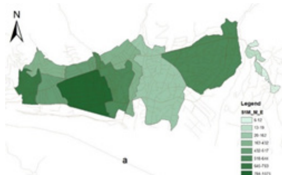
Fig 4: Area of Concrete Moment Frame buildings with extensive damage in different areas of Lavasan city(m2), a: 4 to 8 story, b: 1 to 3 story
