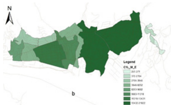
Fig 4: Area of Concrete Moment Frame buildings with extensive damage in different areas of Lavasan city(m2), a: 4 to 8 story, b: 1 to 3 story
