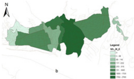
Fig 6: Area of Steel Braced Frame buildings with extensive damage in different areas of Lavasan city(m2), a: 4 to 8 story, b: 1 to 3 story
