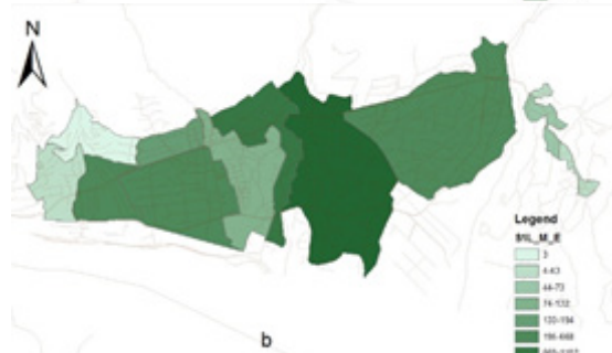
Fig 5: Area of Steel Moment Frame buildings with extensive damage in different areas of Lavasan city(m2), a: 4 to 8 story, b: 1 to 3 story
