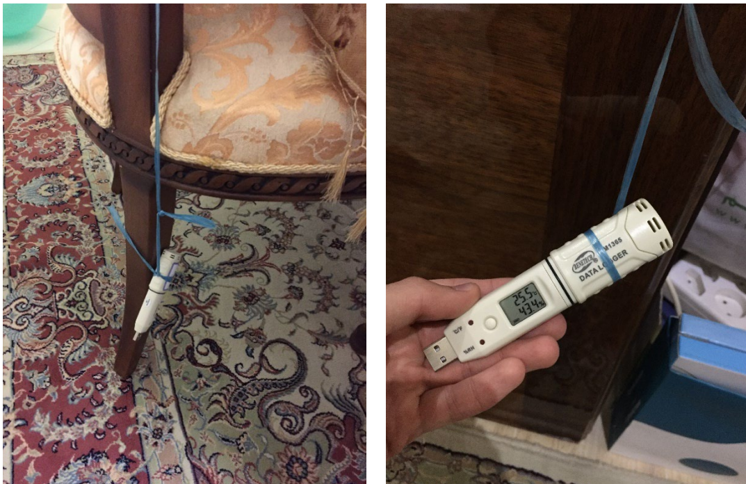
Fig. 5. Data logger for collecting data at both rooms
