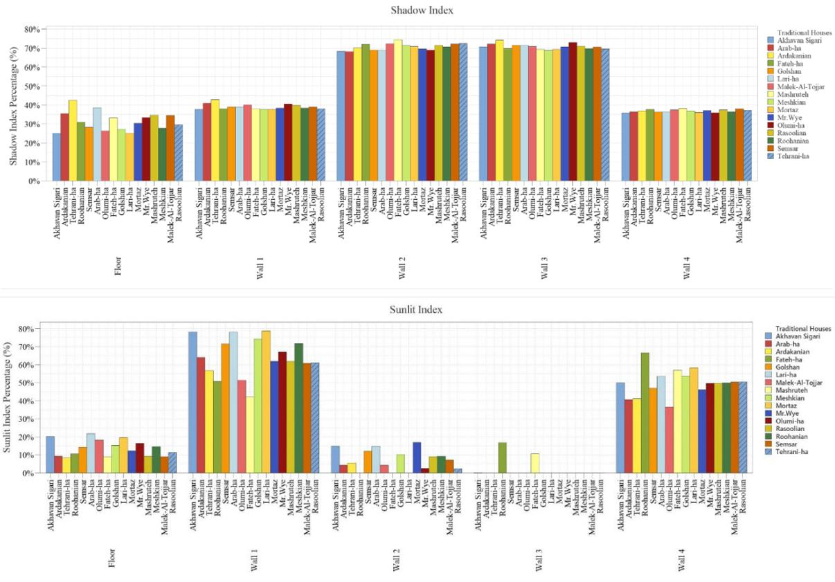
Figure 2: Top) Shadow index on the floor of the courtyard and the surrounding walls on the first day of June, bottom) Sunlit index on the floor of the courtyard and the surrounding walls on the first day of December.
